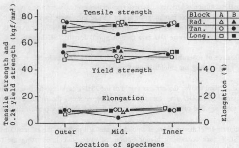
FIG. 3. Tensile properties of the DU ring casting.
