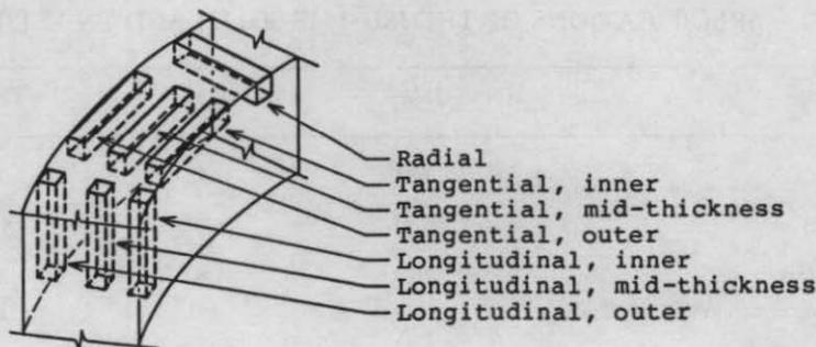
FIG. 2. Locations and directions of specimen cut off from the DU ring casting.
