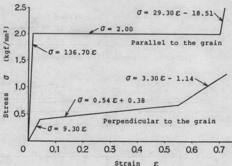
FIG. 7. Dynamic stress-strain diagrams of balsa blocks.
