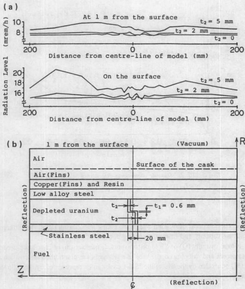
FIG. 6. Influence of gaps between DU rings on shielding performance. (a) Radiation-level distributions, (b) calculation model.
