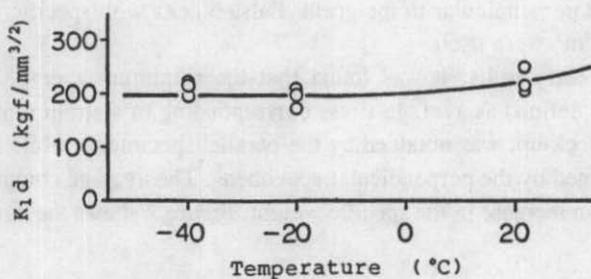
FIG. 5. Dynamic fracture toughness of the DU ring casting.
