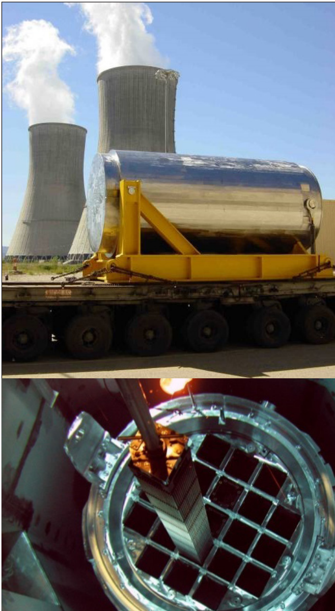
Figure 5. ENSA-DPT dual purpose metal cask
