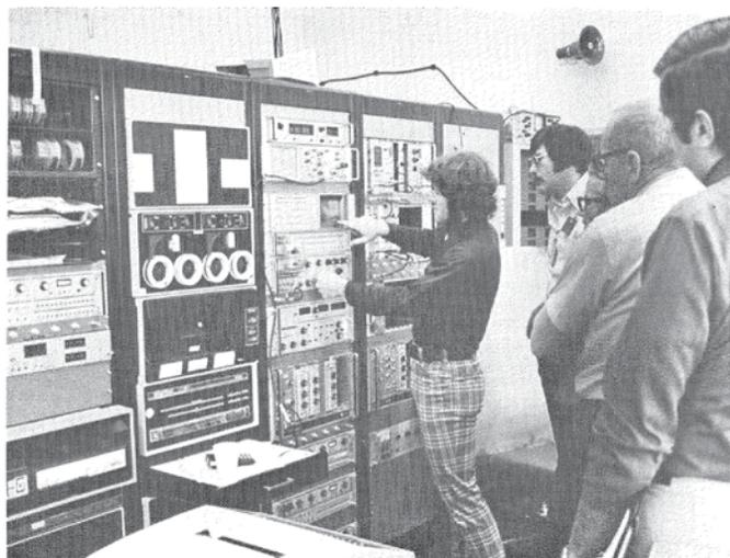
plication to state-of-the-art instrumentation of some of the principles taught in the laboratories, a detailed demonstration of a fully automated segmented gamma scanner [12] is given (Fig. 7).
