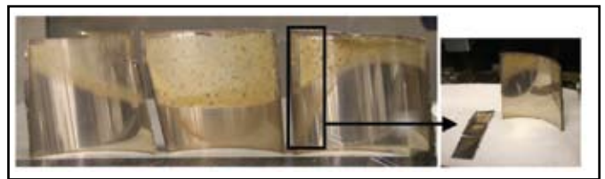
Figure 6. Visual examination photographs from the inside walls of the convenience container: Coated looking surface of convenience container is the headspace region. Sections cut for SEM and EDX examination were taken from region in the box. Portion of coating flaked off during cutting of sample for SEM, as seen in box on left.
