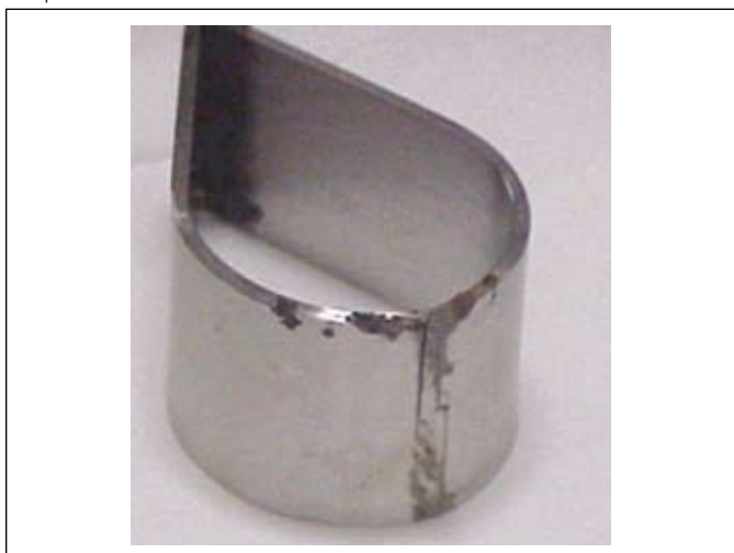
Figure 13. Stress corrosion cracking along the autogenous weld in coupon 304L-20 from container 4a-2
