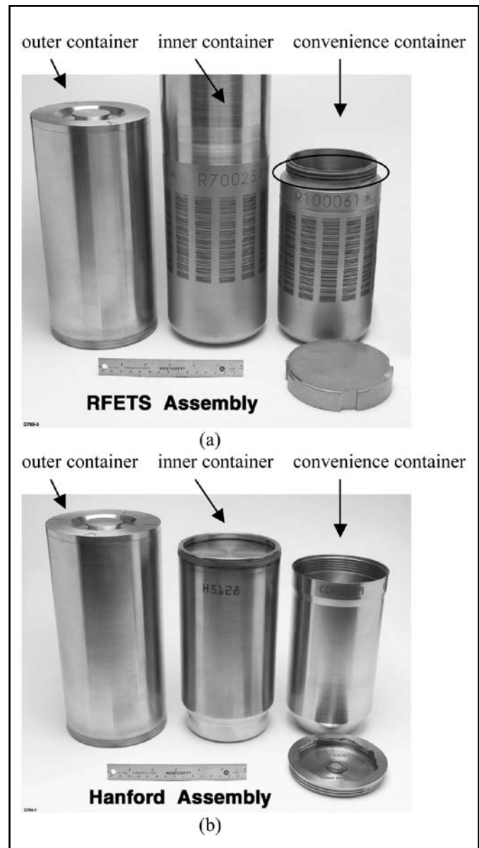
Figure 1. 3013 container configurations (a) RFETS 3013 container. Note silver coated threads on convenience container body (circled). Note: the inner container in Figure 1a is shown prior to cutting to height. (b) Hanford 3013 container. Difference between the two include convenience container design and lid material. Additionally, the inner container body design varied toward bottom of container.
