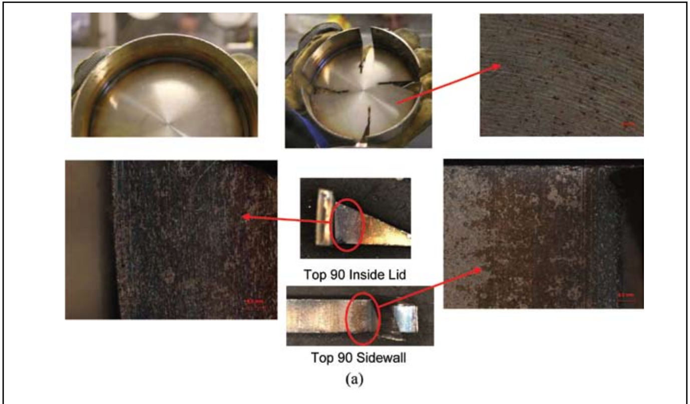
Figure 12. Additional sections from inner container for further analysis during DE. (a) appearance of corrosion particulates and “coating” adhering to surface of lid and side wall. No corrosion depth was seen by SEM. (b) coating product on sidewall likely an iron oxide product with the oxide peak shown in the EDX spectrum at top right. Bottom photo and corresponding spectrum at bottom right shows a chloride peak from corrosion product within incipient pit.
