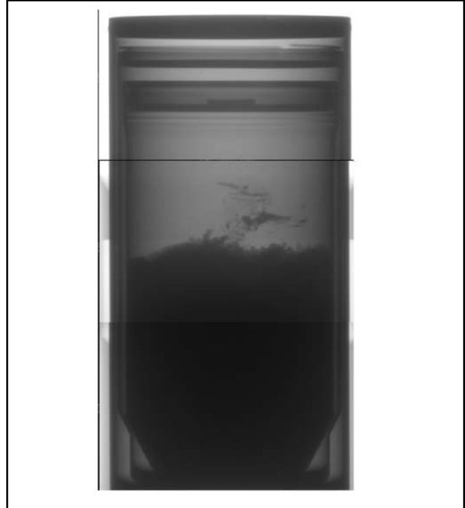
Figure 3. Full can radiography image showing glove
