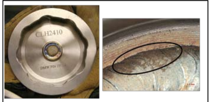
Figure 6. Visual examination photographs from the inside walls of the convenience container: Coated looking surface of convenience container is the headspace region. Sections cut for SEM and EDX examination were taken from region in the box. Portion of coating flaked off during cutting of sample for SEM, as seen in box on left.
