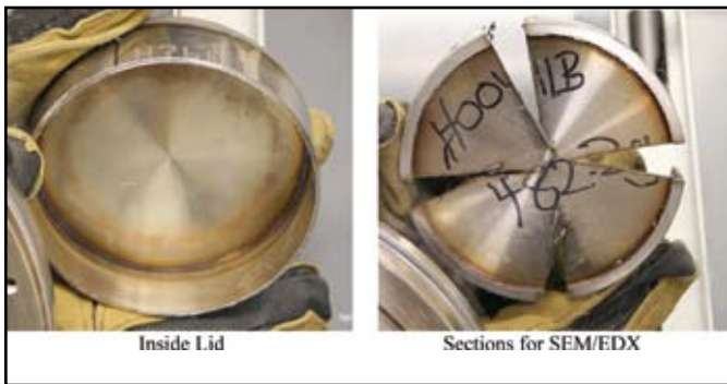
Figure 14. Sections cut from inner container for SEM and EDX analysis
