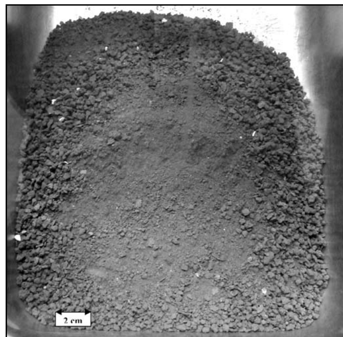
Figure 2. Sample H001992 after removal from the 3013 inner can. The small [blue and] whitish flecks are indicative of material that might be sampled and designated as 'if required' samples. This material contains approximately 52 percent actinides by weight.
