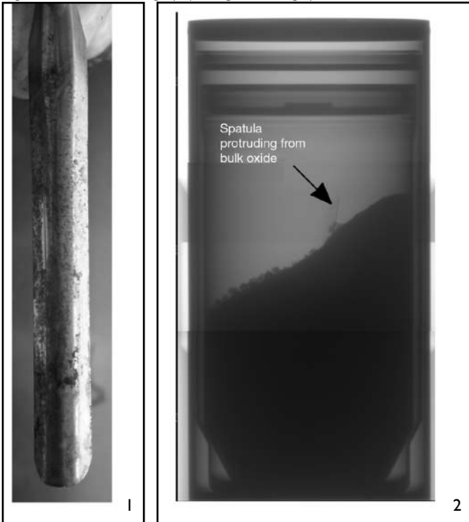
Figure 2. Full can radiography image showing spatula
