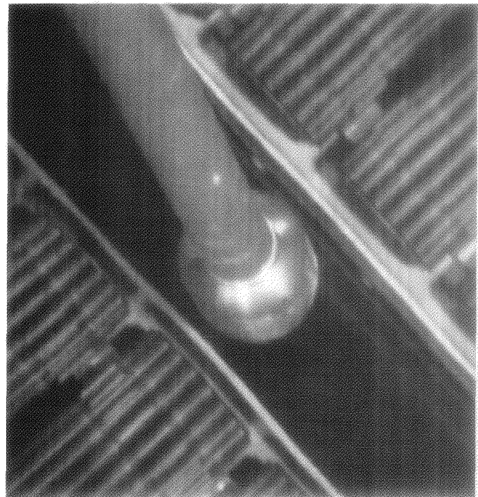
Figure 2. Photo of SCAV detection head and spent CANDU fuel bundles in storage rack of pool
