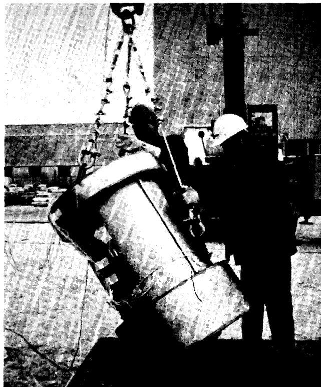
Figure 11. Scale model of CIC with impact limiters before drop test
