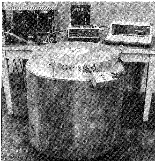
Figure 7. The "Neutron Multiplicity Counter" in operation at the Los Alamos safeguards R&D laboratory. The outer shield is ~ 80 cm diameter by ~ 70 cm high, and the central sample cavity is 15 cm in diameter.
