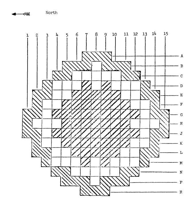
Figure 2 Initial Fuel Loading for San Onofre Nuclear Generating Station, Unit 1
