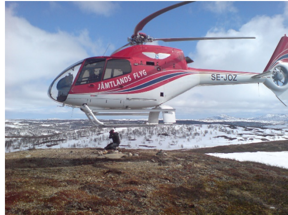
Figure 11. Example of rolling shutter temporal distortion in an image of helicopter blades. 11
