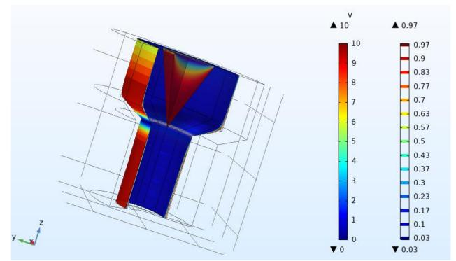
Figure 9- Iso Surface Phase Indicator from Phase 1 to Phase 2, and electric potential 3 D distribution.
