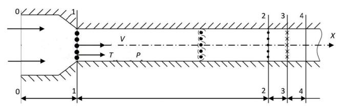
Figure 2- System of the reactor for dispersed combustible aqueous organic composition for treatment using plasma [1].
