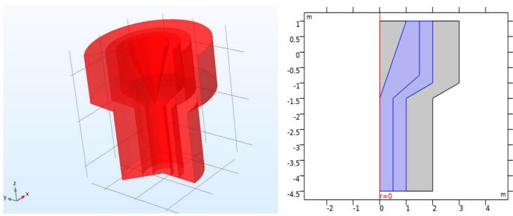
Figure 3- DC thermal with specific domains for Arc plasma flow and Uranyl Nitrate solution. Plasma Plant 3D Distribution, and 2D Plan [6].
