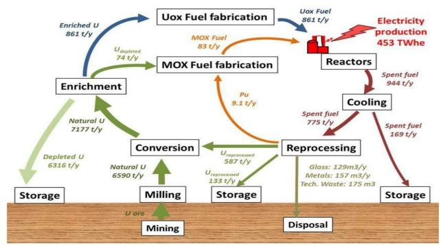
Figure 1- Detailed diagram of the PUREX process [2].
