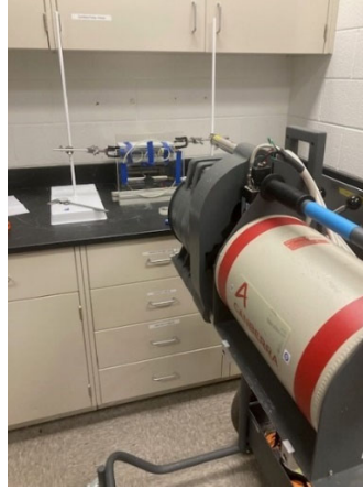
Figure 55. The BEGe detector and the leaded glass were setup to allow measurement of the source tubes through the leaded glass and the various small openings.
