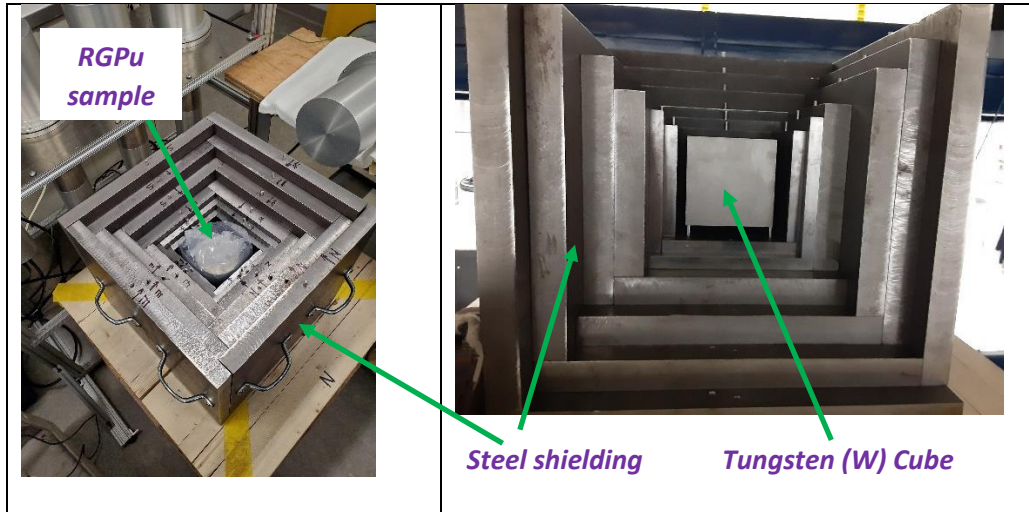
Figure 1: Mock-up used for neutron/gamma-ray measurements (left) and muon scattering experiments (right). Front and top layers removed to show inner samples.
