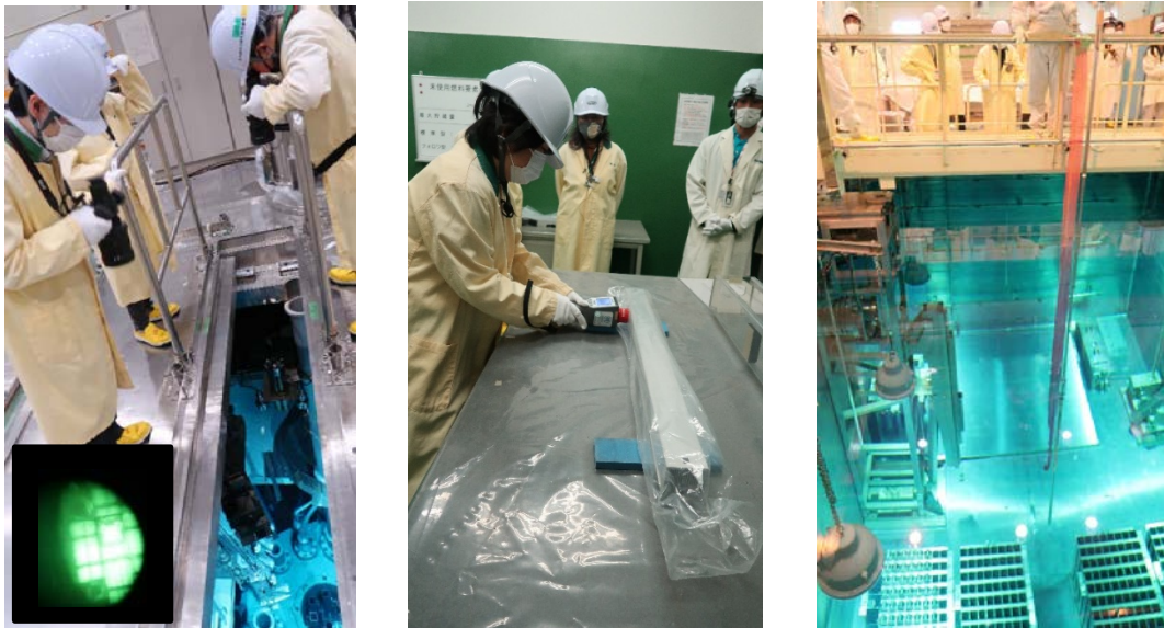
FIG. 11. Exercise on ICVD at reactor core, HM-5 using fresh fuel, and underwater NDA measurement at the spent fuel pond.
