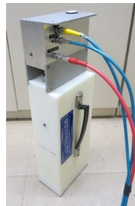
FIG. 2. Handy-type He-3 detector.
