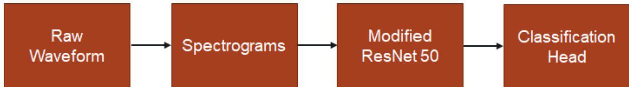
Figure 4. Block diagram of the data to classification pipeline
