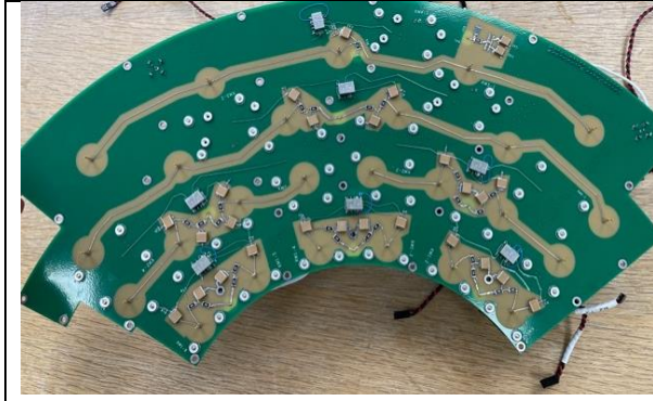
Fig 4 Left: bottom view of R2 HV distribution board
