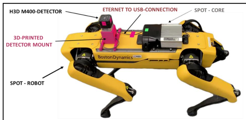
Figure 2. H3D M400-Detector integrated with Spot, Spot-Core system
