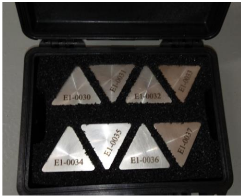
Figure 3: Eight ^{233}\text{U} oxide triangles in case
