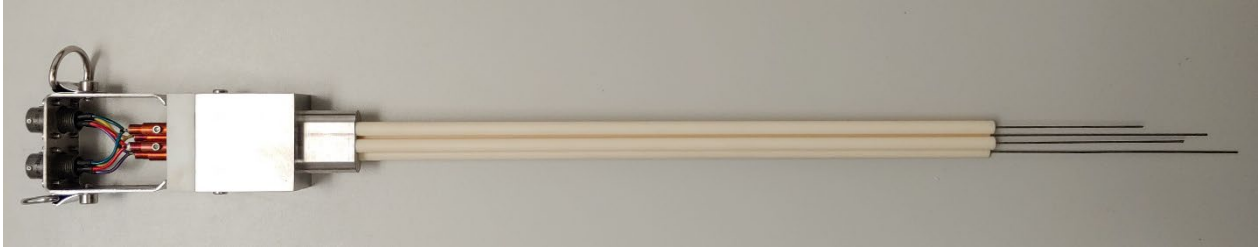
Figure 3. Multielectrode array voltammetry sensor
