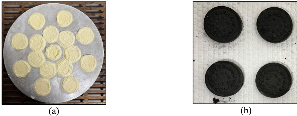
Figure 3: Images of the pre-cure molded filters (a) and the carbonized, hydrophobic filters (b).
