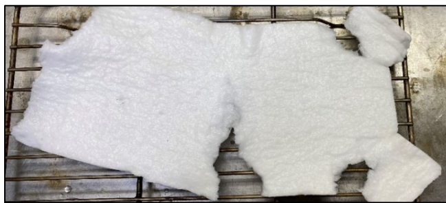
Figure 1: Image of a sheet of saturated fiber that was ripped during handling.
