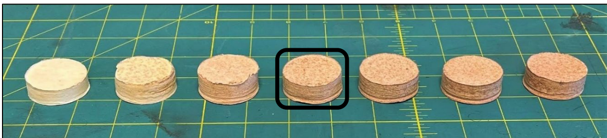
Figure 7: Images showing the results of different resin curing times with the selected curing time highlighted in black.
