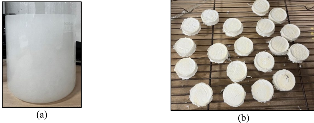
Figure 2: Images of the fiber slurry (a) and the molded, unbonded filters (b).
