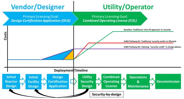
Figure 3. Comparing traditional security approaches to the proposed SeBD approach using a regulatory/engineering lifecycle model, recreated from [2]
