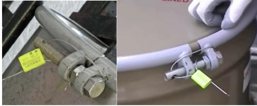
Figure 2-1. Pull-tight TID on CCO
