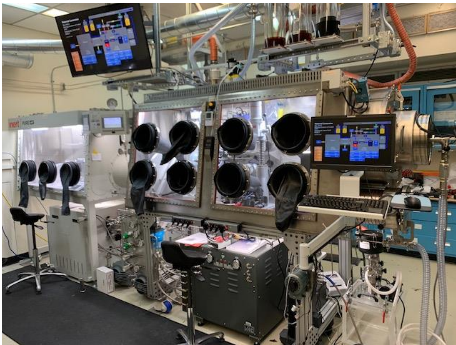
Figure 3. Inert glovebox for evaluating, stabilizing, and repackaging air-reactive material.
