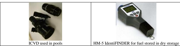
Figure 10 – Main verification devices used by Euratom in EDF NPPs. © *EDF*
