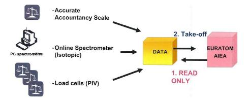
Figure 8 – Georges Besse II Data acquisition for Safeguards.
