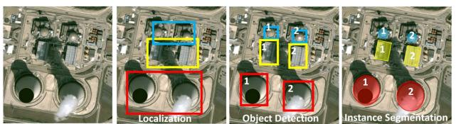
Figure 3. Illustration of localization, object detection and instance segmentation of different components of the nuclear power plant shown in Fig. 2. Red highlights cooling towers, yellow outlines turbines, and blue outlines reactors. Numbers represent IDs of individual instances of cooling towers, turbines, and reactor buildings. Image credit © Google Earth.
