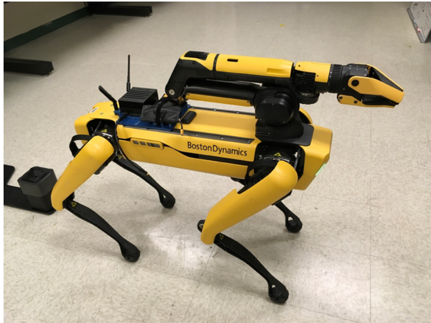
Figure 1: Spot carrying a custom-built Nvidia Xavier mount.
